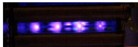
(Fig 2.2) Image of the corona discharge creating EHD thrust on a MAIE prototype in late July 2023.
