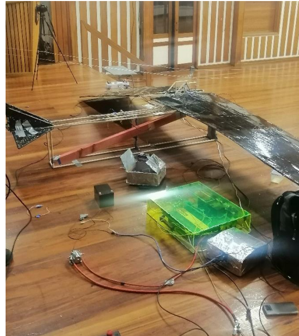
(Fig 2.13) Shows the launcher during testing, with the aircraft on top of the launcher.
