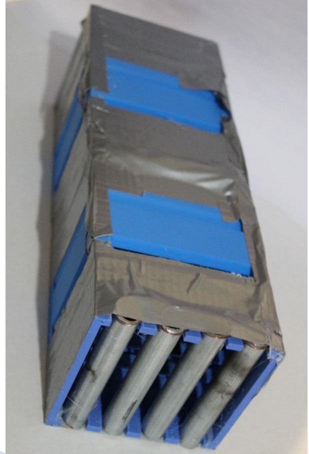
(Fig 2.6). Image of the constructed 3 module MAIE
