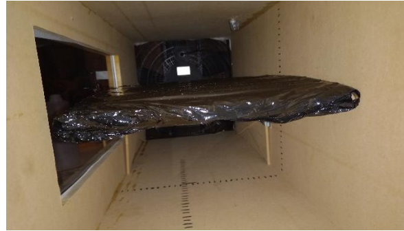
(Fig 2.11) This is the wing within the wind tunnel during testing.
